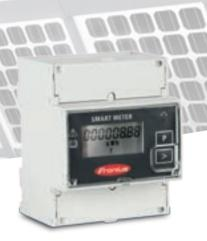
The Fronius Smart Meter is a bidirectional meter which optimises self-consumption and records the household's load curve. Thanks to highly accurate measurements and rapid communication via the Modbus RTU interface, dynamic feed-in control when feed-in limits are imposed is faster and more accurate than with the SO meter.
