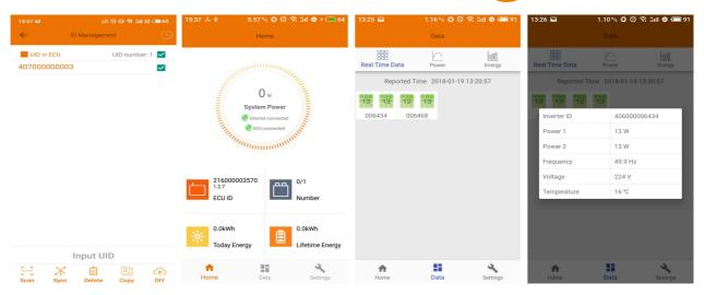
6: Configure IDs, date, Network Connection and WLAN connection.
