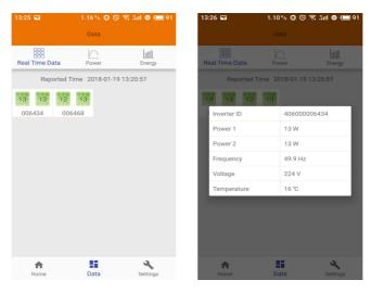
Green panel indicates the inverter is successfully connected.
