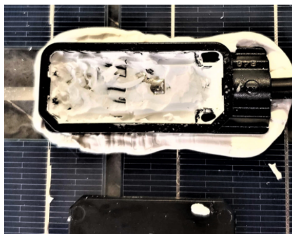
The junction box above became unsealed after damp heat testing.
